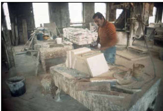
A view of the Gladding McBean & Company plaster shop where molds, used in the manufacture of terra cotta, are produced.
