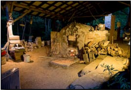
Anagama kiln, Japanese-style wood-firing kiln Photo by Richard Wanderman
